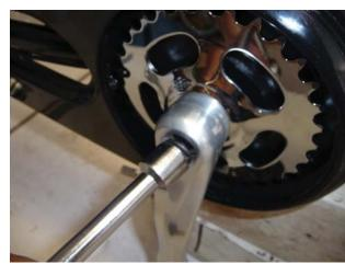
Assembling chain, piece of iron wire, wire in chain guard, hook chain and pull through the chain guard, spin the chain with chain wheel, hook wire and pull back.
