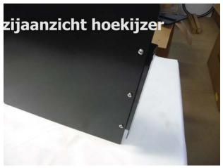
Assembling, assemble both angle irons, placing side of the barge, assemble both sides, secure the bolts and mucks by hand
