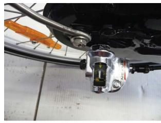
Adjust the gears, put the gears in the second stand, and place the yellow spot between the two stripes, adjust the bolt to place the yellow spot between the stripes
