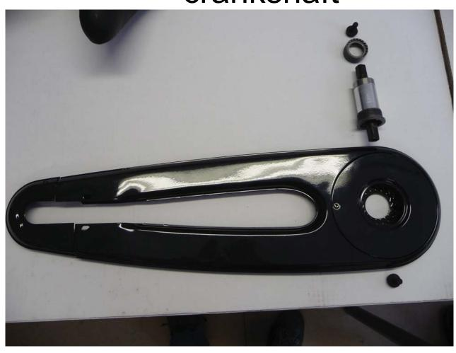
Remove for assembling, slide chain guard over the cable and frame tube assembling the crankshaft, crankshaft, secure anti-clockwise with the supplied wrench secure anti-clockwise and other side clockwise
