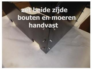
Assembling, angle iron front side with more than 90 degrees, inside barge 020 front side, secure the bolts and mucks by hand, watch for the skew side.
