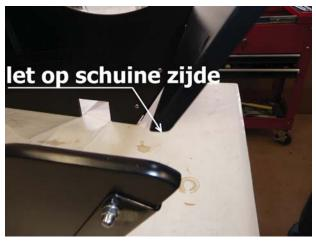
Sequel of assembling, turn barge upside down, place some nails on the corners through the bottom in the sideboards, screws for the bottom, place all screws on the sole plate, be careful with bursting of the sideboards
