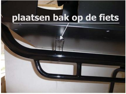
Sequel of assembling, secure the barge with 4 bolts and locknuts, secure the barge to the steering tube
